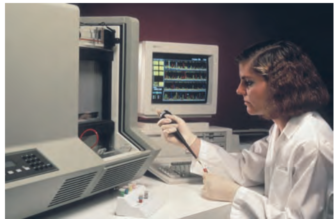
Figure 1.3 An automated DNA sequencer. This instrument can sequence about 1,000,000 base pairs a day and newer technologies are 100 to 1000 times faster.
